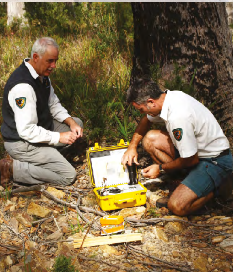
Ranger Mike Smithson and Fire Management Officer Paul Black, Parks and Wildlife Service, Tasmania, Australia, measuring fire fuel humidity levels as part of planning for fuel-reduction burns Source: Graeme L. Worboys
